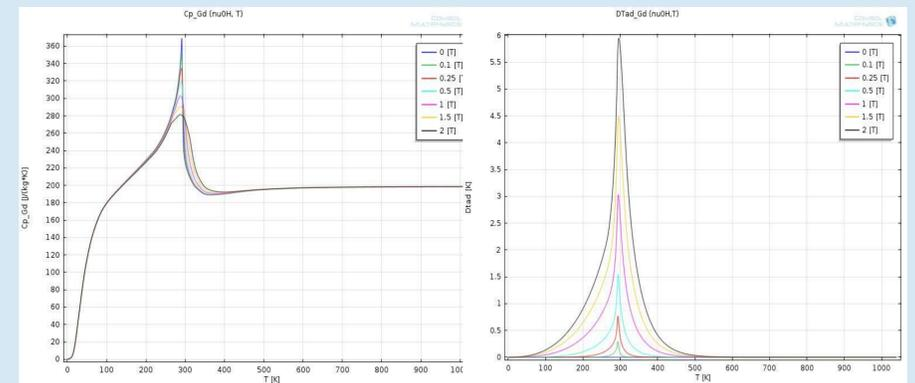
**Figure 4.** Interpolation of values of specific heat of Gd  $C_p(T, \mu_0 H)$ , and adiabatic temperature difference of Gd  $\Delta T_{ad}(T, \mu_0 H)$ , using COMSOL function “interpolation”
