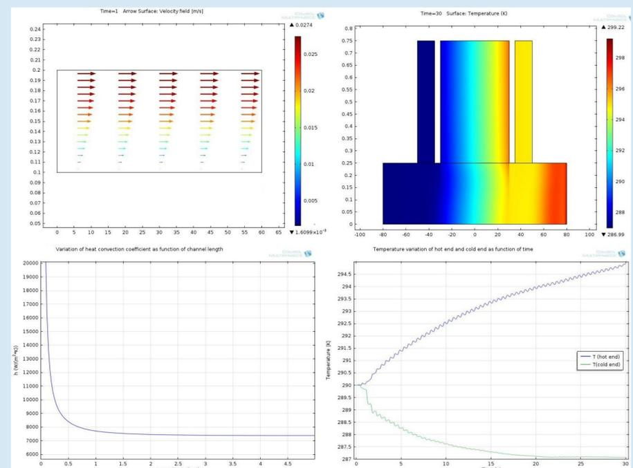
**Figure 5.** Representation of velocity field, temperature field, heat transfer coefficient variation, cold end and hot end temperatures variation
