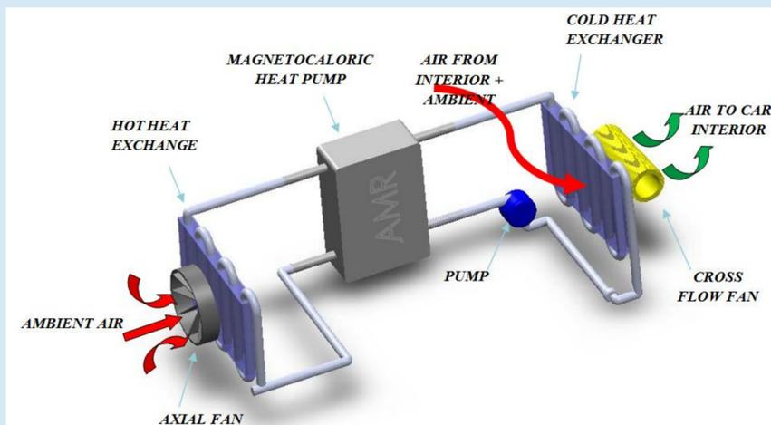
**Figure 2.** Scheme of Magnetocaloric heat pump integration in air conditioning circuit of electric vehicle
