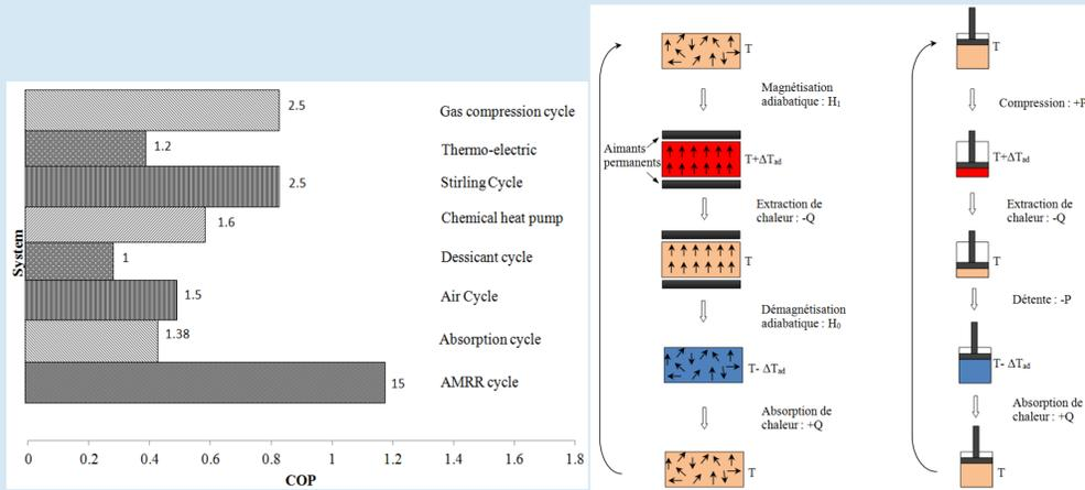
**Figure 1.** a) Comparison of principal refrigeration systems performance b) MCE and comparison with a vapor compression cycle
