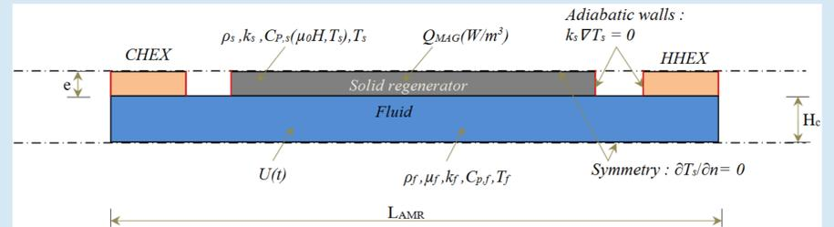
**Figure 3.** Physical model of an Active Magnetic refrigeration cycle
