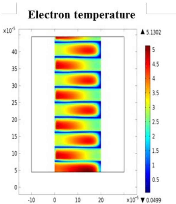
**Figure 1:** Electron temperature distribution
