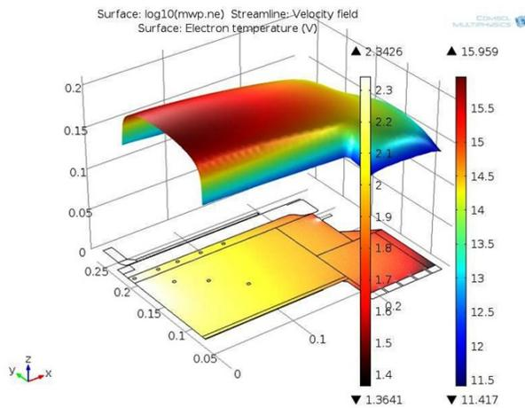
**Figure 3:** Log of plasma density and electron temperature in Ar+H<sub>2</sub> plasma at 35 mTorr.
