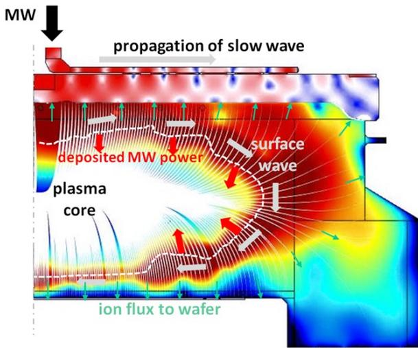
**Figure 2:** A comprehensive view on processes occurring in RLSATM PECVD reactor. Color range for individual parameters was artificially emphasized to expose the physics inside reactor.
