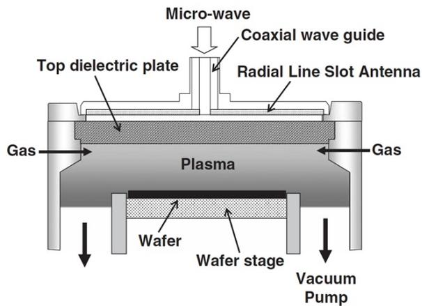
**Figure 1:** A cross-sectional view of RLSATM PECVD reactor.
